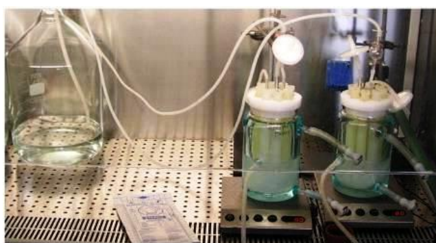
Two CDC biofilm reactor vessels coupled to a bottle with fresh medium. (Coenye and Nelis, 2010)
