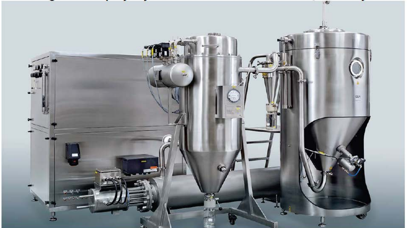
Figure 67 : Spray dryer MOBILE MINOR™ from GEA, Germany
