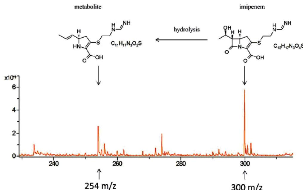
**Figure 1. MALDI-TOF MS analysis of imipenem.** (A) Imipenem and its natural degradation product. (B) Mass spectra of imipenem and its natural degradation product as determined using the Ultraflex mass spectrometer.
