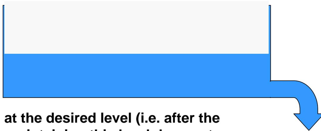
once a bath is at the desired level (i.e. after the loading dose), maintaining this level does not depend upon its volume but of the ratio of tap and drain flows (which must be equal: in = out...)
